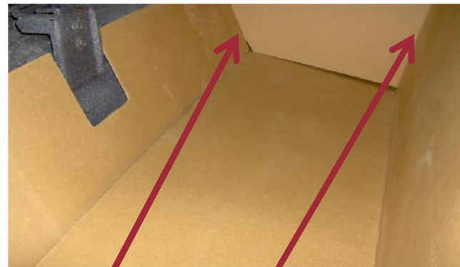
There may be enough clearance on the panels and will fill in once all the upholstery is in place. You may need to sand to fit precisely.
