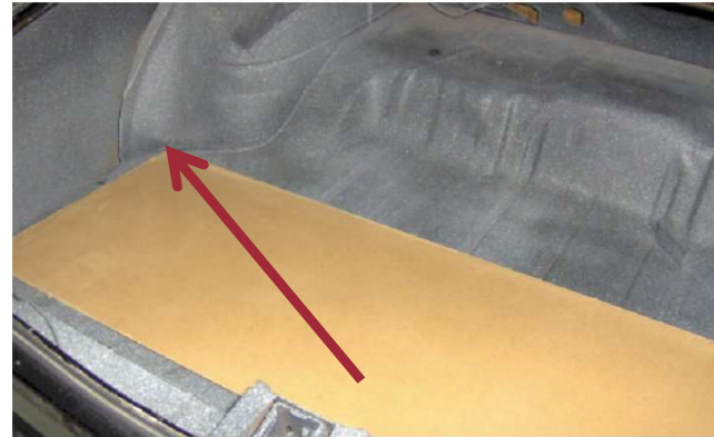
The first piece is the floor and should fit against the bottom of the fender well on both sides.
